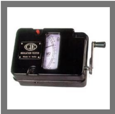
Portable Insulation Tester
