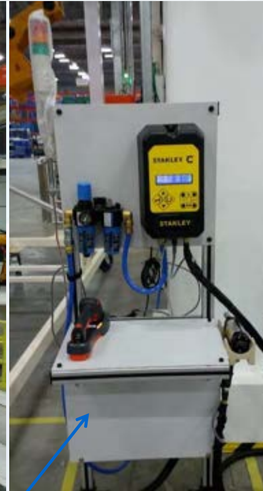
Main Control Panel housing PLC, PC & SCADA
