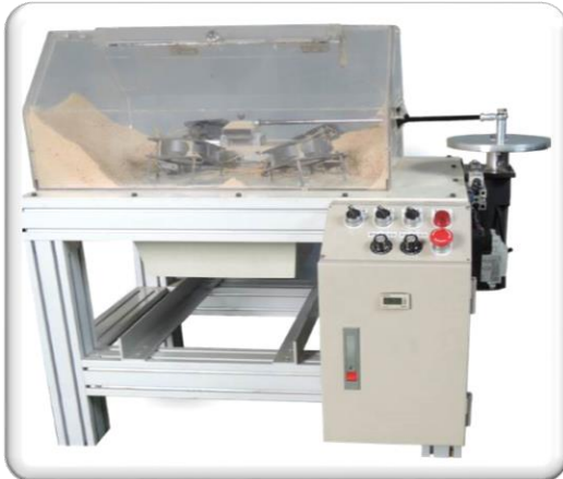
Sealing Test in harsh environment
