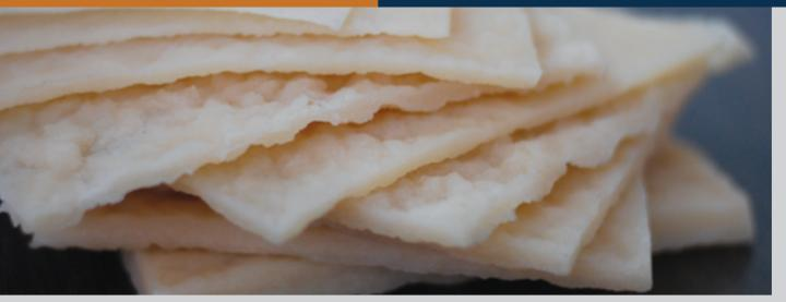
**NBR-PVC**, as the name suggests is a combination or blend of acrylonitrile butadiene rubber (nitrile rubber/nbr) and polyvinyl chloride (pvc resin) and is categorised as a 'polyblend'.
