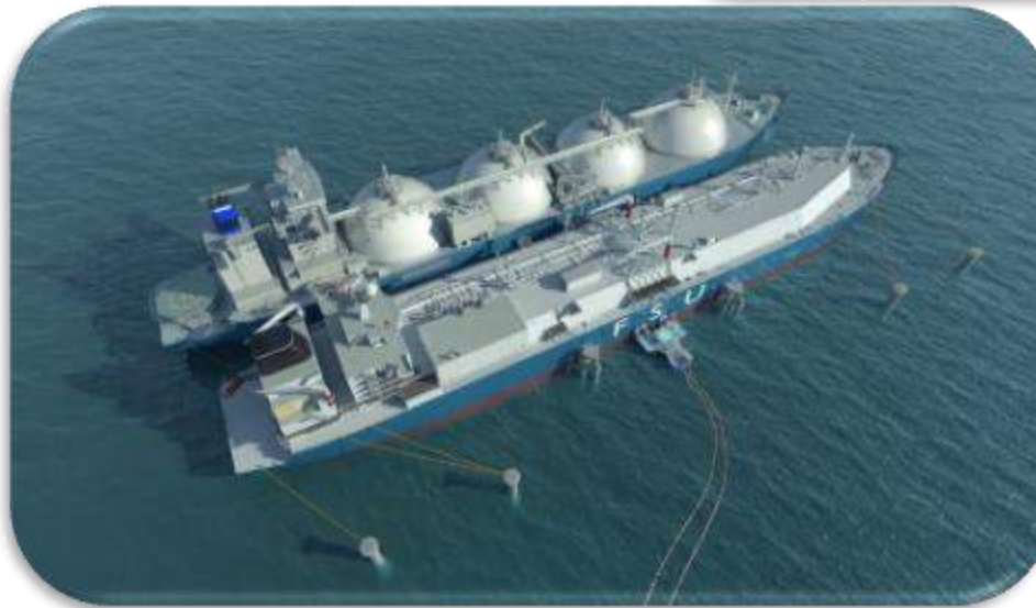
Jetty less Regasification Terminal (Floating Hose Technology)
